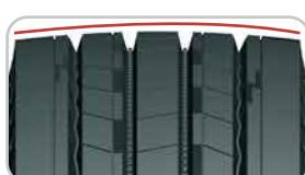
Wide driving surface and deep groove design ensure ultra-wear resistance.
